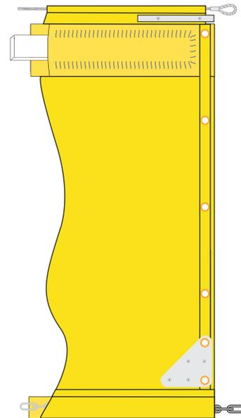
**NOTES:** Depth measured from top of flotation device to bottom of curtain. Specified fabrics will be supplied per order: Permeable and non permeable. Buoyancy increased when specified. Ballast chain increased when specified.
