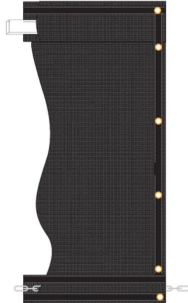
**NOTES:** Depth measured from top of flotation device to bottom of curtain. Specified fabrics will be supplied per order: Permeable and non permeable. Buoyancy increased when specified. Ballast chain increased when specified.
