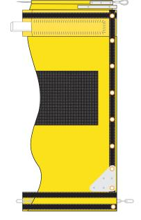
**NOTES:** Depth measured from top of flotation device to bottom of curtain. Specified fabrics will be supplied per order: Permeable and non permeable. Buoyancy increased when specified. Ballast chain increased when specified.
